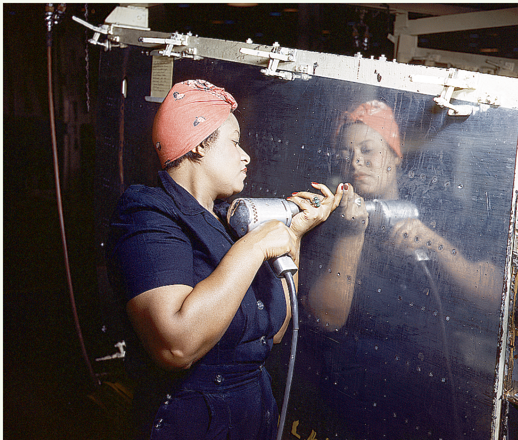
In 1943, a real-life “Rosie the Riveter” operates a hand drill at Vultee-Nashville, Tennessee, working on an A-31 Vengeance dive bomber.
